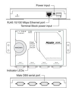
**Reset Button**—The reset button is used to load factory defaults. Hold the reset button down for five seconds using a pointed object such as a straightened paper clip. Release the reset button when the Ready LED stops blinking.
